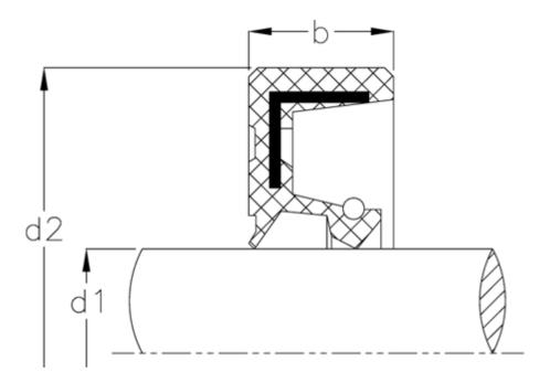
$\begin{array}{ll} b & = 12 \\ d1 & = 135 \\ d2 & = 170 \\ Material = NBR \end{array}$
